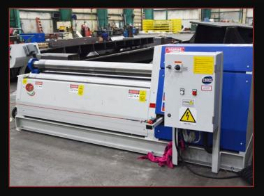
Our Parmagiani 4-roll machine can roll a 1"x 10' (Thicker if less width).
